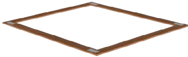
2 No. 38 x 86 Gang-Nail Plates pressed into both faces at each corner
